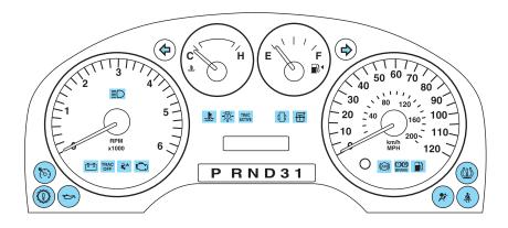
Warning lights and gauges can alert you to a vehicle condition that may become serious enough to cause extensive repairs. A warning light may illuminate when a problem exists with one of your vehicle's functions. Many lights will illuminate when you start your vehicle to make sure the bulb works. If any light remains on after starting the vehicle, refer to the respective system warning light for additional information.
